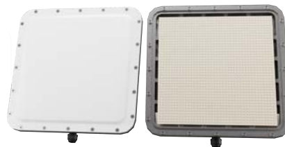
Figure 3. RIS 28G. (Left) w/ Radome. (Right) The Reflection Elements.
