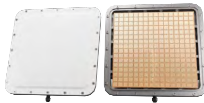
Figure 3. RIS 4G7. (Left) w/ Radome. (Right) The Reflection Elements.
