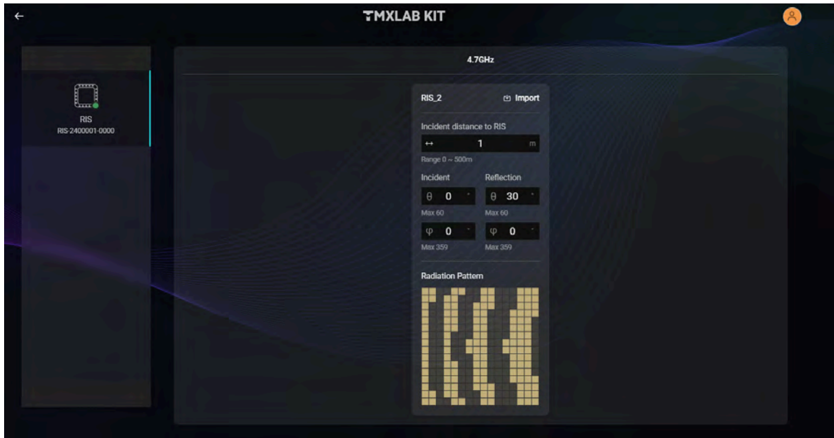
Figure 6. TMXLAB Kit - Software GUI for controlling XRifle Dynamic RIS.
