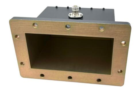
WR650 Waveguide to Coax Adapter Frequency: 1.13-1.73 GHz Flange: FDP14 (Cover) = UDR84 Connector: N-female
