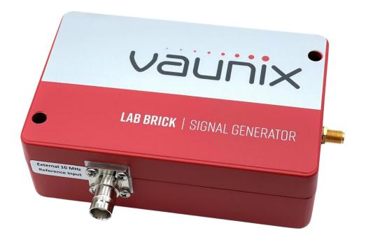
Wireless Testing USB powered and controlled Selectable internal/external 10 MHz reference Robust aluminum construction Programmable frequency stepping Portable LO Source Phase-continuous frequency sweep (LFM) Operate multiple devices directly from a PC or self-powered USB hub Includes easy to install and operate GUI High-speed internal and external pulse modulation High-speed switching up to 20 GHz Easily programmable for ATE applications Customization available for unique requirements
